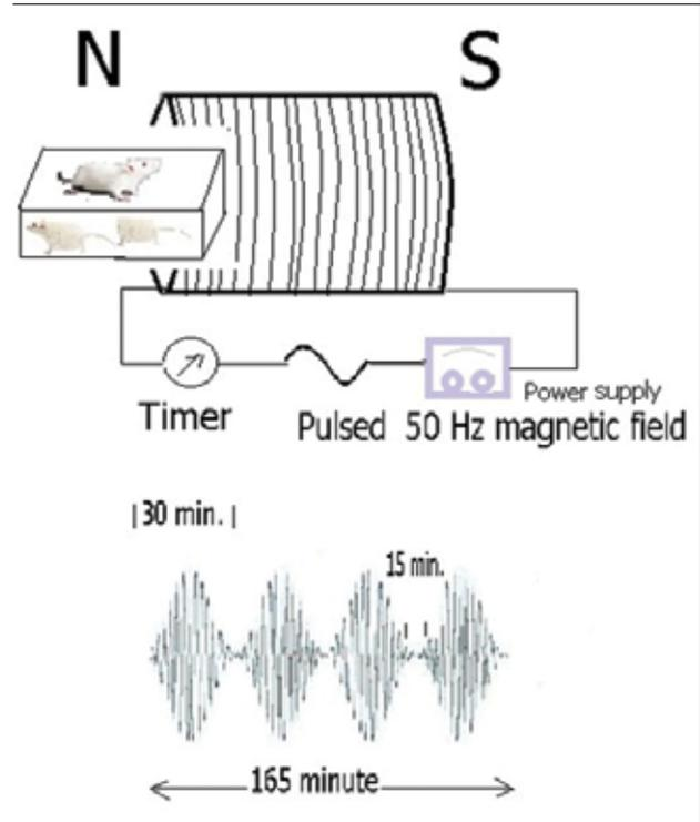
Figure 2. a-c. Experimental set up (a, b, c) for MF strengths (1, 5, and 10 mT). The solenoid was powered by a power supply
