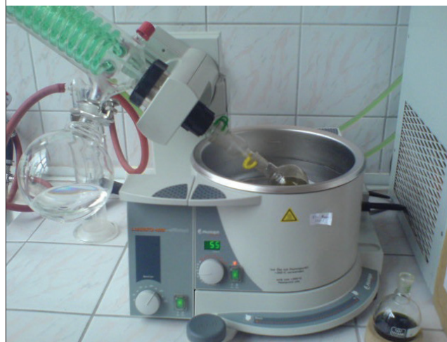
Figure 1. Removal of ethanol by an evaporator after filtration (Evaporator, Heidolph Laborota 4000, Germany)
